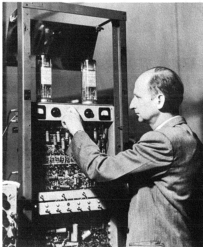
Dynamic life test equipment for SB-256 storage tubes.
